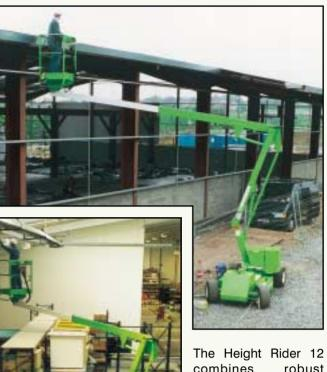
The Height Rider 12 combines robust construction with compact, low weight design. The Bi-Energy option allows it to work for extended periods inside and outside making it the perfect allrounder.
