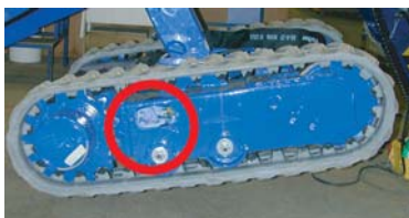
Fig. 66a Niplerne for strammerullen sidder her.
